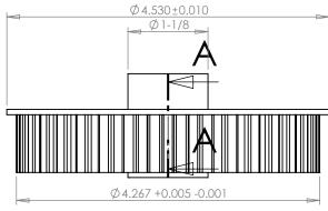
**NOTE: CORED PULLEYS** HAVE 1/16" THICK RIBS, REINFORCEMENT
